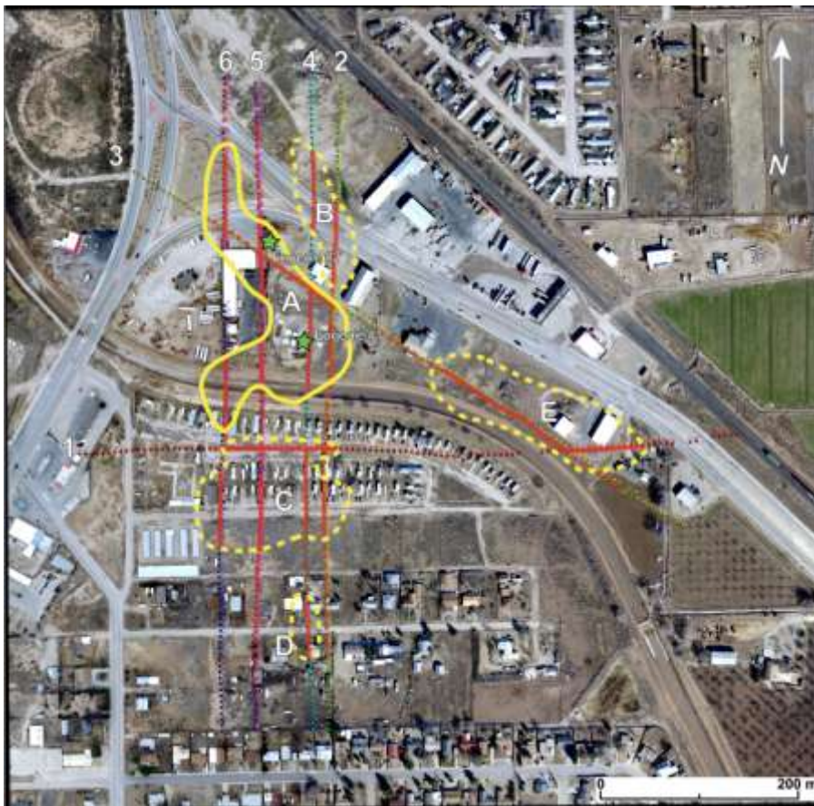
Map showing locations of possible subsurface cavities in Rustler and Salado formations. Solid red highlighted lines indicate areas of probable cavity formation. Dashed red lines show areas of possible brine-saturated breccia. The area outlined by a solid yellow line is probably underlain by a solution cavity; dashed yellow lines are areas of low resistivity.
